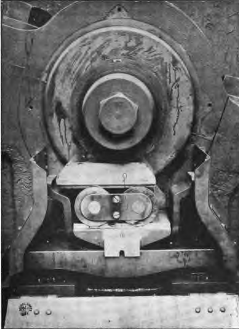
ANTI-FRICTION BEARING OF THE 280-MM. GERMAN GUN MOUNT.
